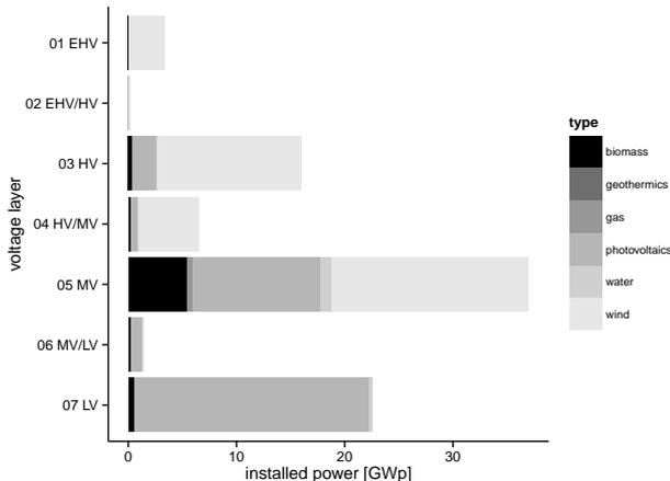
Fig. 2. Types of renewables installed in the layers of the electrical grid in Germany [3]; EHV = Extra High Voltage, HV = High Voltage, MV = Medium Voltage, LV = Low Voltage
