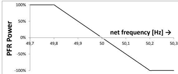
Fig. 5. Characteristic Curve for calculating PFR Power Demand
