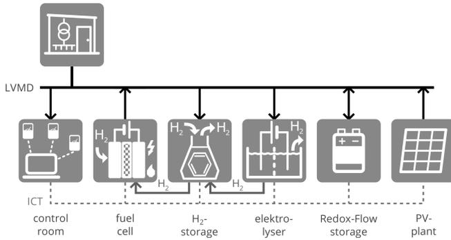
Fig. 3. Electrical and communication structure of the test centre; LVMD = Low Voltage Main Distribution, ICT = Information- and Communication Technology
