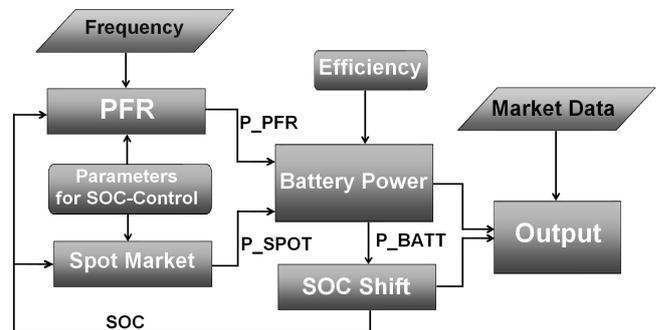
Fig. 4. Simplified simulation scheme
