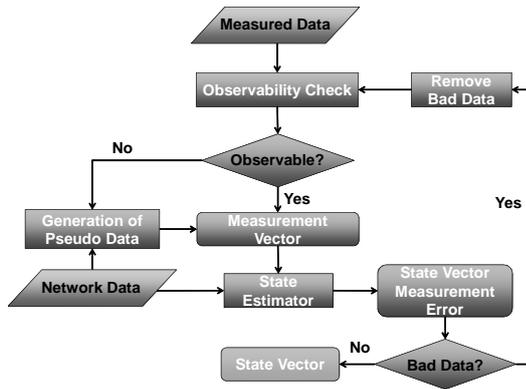
Fig. 7. Procedure of a State Estimation with compensation of missing measurements
